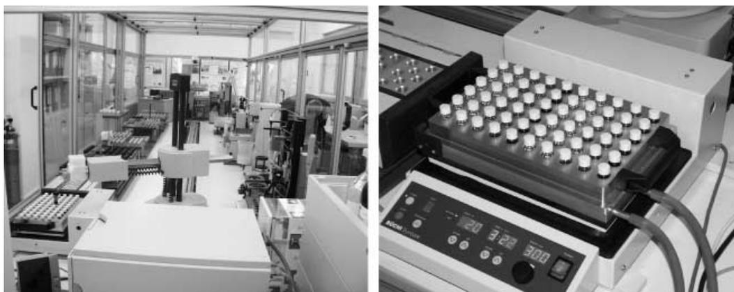
Figure 1. Zymate laboratory automation system (left) and 60-well Syncore reactor station (right).
